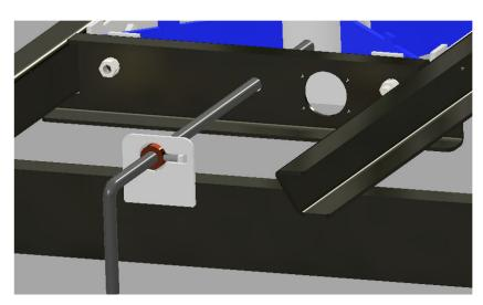
Slide the locking collar with the long set screw and the mounting plate up close to the handle and slide pull pin above the frame rail and through the guide hole and into the receiver. Line up the mount plate to be centered around the lock collar and clamp the plate in place. Weld the plate in place and
