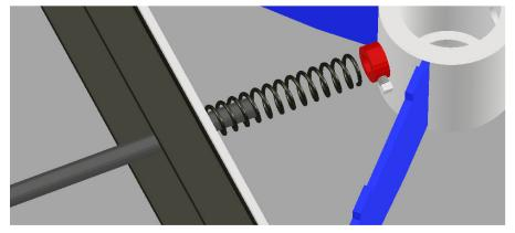
Pull the pin back far enough to slide on the springs and the lock collar with the short set screw, and Push the pin back into receiver.
