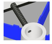
Pull the pin just far enough to let it Release the 5<sup>th</sup> wheel ball and slide The lock collar with long screw up to The mount plate and tighten it down With the set screw down in line with the handle. Slide the pin back into The receiver make sure it goes
