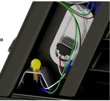
Logic Box – On bale beds only behind the top drivers side headache light there is a logic box for the center brake light. The logic box filters out the turn signals – ( yellow and green wires) if the center light blinks then you may have to replace the logic box. If installed on an older pickup that has the 3 wire brake and turn signal setup read the (ORANGE WIRE) and follow instructions on how to bypass the logic box.
