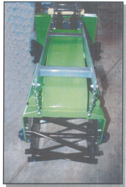
The unique design of the floating row unit catches the debris thrown from the disc and funnels it into the rolling basket.
